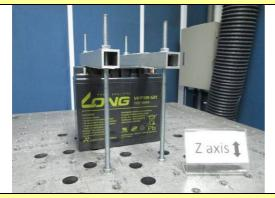
5. Vibration Test: Z axis Pressure Differential Test
